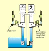
Solution level below impeller with priming tee. Check valve and throttling valve
