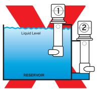
In Tank - Solution may pour out of weep hole during  $\mid$  Non-flooded conditions. Pumps will not pump operation
