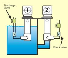
Solution level above impeller. Suction head available
