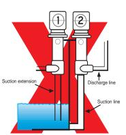
Solution level below impeller. Pumps will not pump
