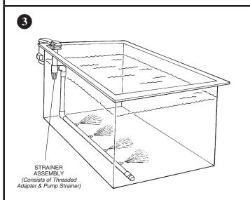
Example shows BXL2500 with over-the-side motor and single pipe positioned near tank wall to provide side-to-side motion. Important: Strainer assembly must be used to prevent foreign objects from being sucked up into and damaging impeller when <u>any</u> FLO KING pump is used without filter cartridge (for agitation only).
