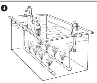
For very aggressive agitation or for large tanks, two pumps can be employed. As a rule when using the BX1200 with piping, use a 3/4-to-1" reducer fitting on the pump discharge port and 1"-diameter vertical and horizontal pipe. For the 2500, 3000, and 5000-series models, use a 1-to-1-1/2" reducer fitting on the discharge port and 1-1/2"-diameter pipe. For the SP12K, use a 1-1/2-to-2" reducer fitting and 2"-diameter pipe.
