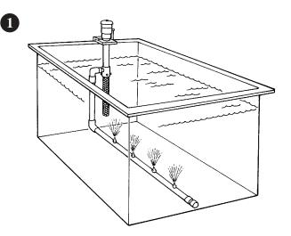
**FLO KING** BX1200 system with single pipe and Floductors<sup>TM</sup>. Pump can be pivoted at threaded 90° elbow and leaned back to change filters. Floductors<sup>TM</sup> are inexpensive, take up little tank space, and are easily installed with hand drill and tap.
