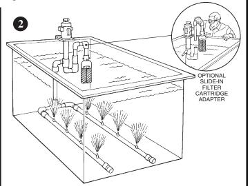
Where required, two pipes of same length can be used without reducing agitation. Optional Slide-in Filter Cartridge Adapter (SIFCA) enables filter changes without moving pump from tank and without disturbing sparger pipe.
