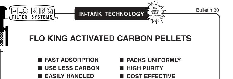
**FLO KING** pelletized carbon is preferred over granular and powdered carbon because it is easier to handle and its unique size and shape allow for uniform mechanical packing and little flow restriction. This results in faster, more thorough adsorption of organic impurities.
