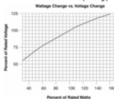
Wattage varies as the square of the voltage. Graph on the left provides a quick method of finding the percent change in wattage caused by operating at various percentages of rated voltage. Heaters are designed to have a give wattage output at a specified voltage and operation at other voltages affects the wattage output considerably. The following ratio can also be used.
